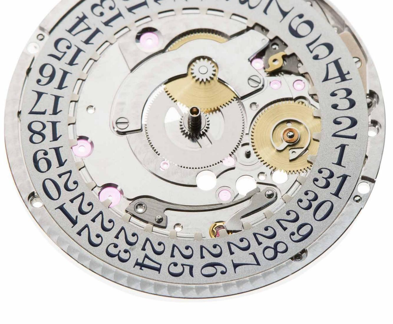
The cover plate for the calendar mechanism removed. This plate both guides the calendar disc and holds in place the indexing pawl.
